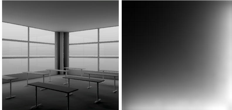
Figure 61: Daylight factor values in the initial situation
