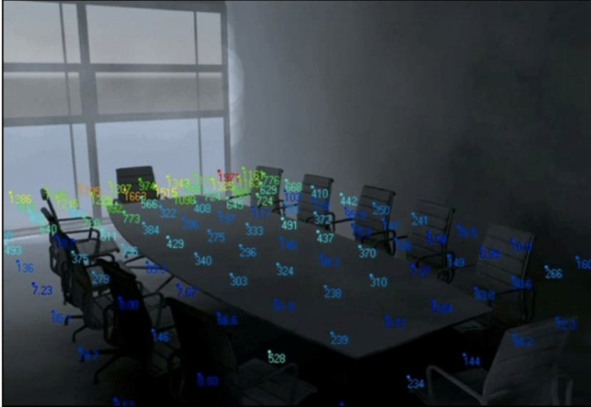
Figure 9: Example of the results obtained with 3DSMaxDesign (illuminance values)
