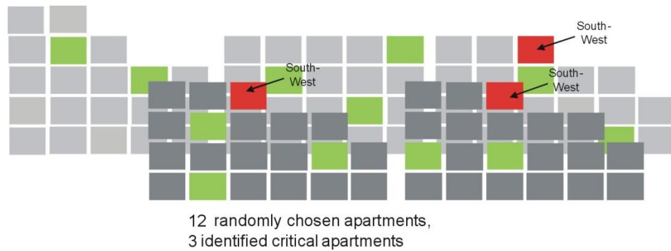
Figure 5-13: The green marked apartments are selected randomly, the red ones identified to be necessary for measuring the critical zone.
