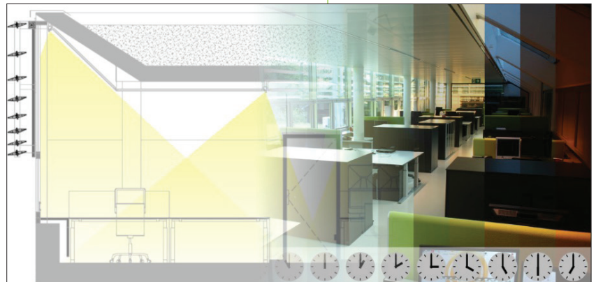
▲ Schematic design of integrated daylighting and electric lighting solution, and example sequence of interior lighting conditions in the report's design project at the Bartenbach R&D office in Austria.
