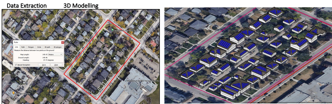
Figure 49: Example of data extraction and measurements using Google Earth and identifying suitable surfaces for PV installations
