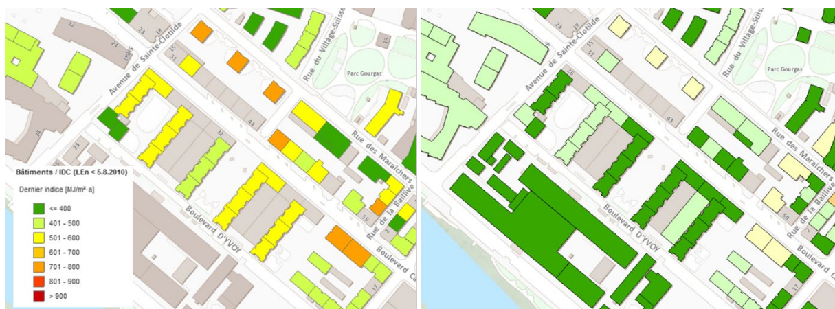
Figure 58 : Measured heat index (in MJ/m 2 /year) before the renovation (left) and after the renovation (right) (source: SITG)
