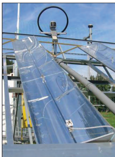
Three of the 12 process heat collectors that were developed or investigated within SHC Task 33. Round Robin tests were carried out at three test centers in Germany and Portugal.
