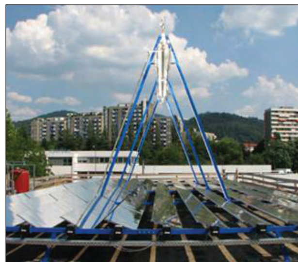
Three of the 12 process heat collectors that were developed or investigated within SHC Task 33. Round Robin tests were carried out at three test centers in Germany and Portugal.
